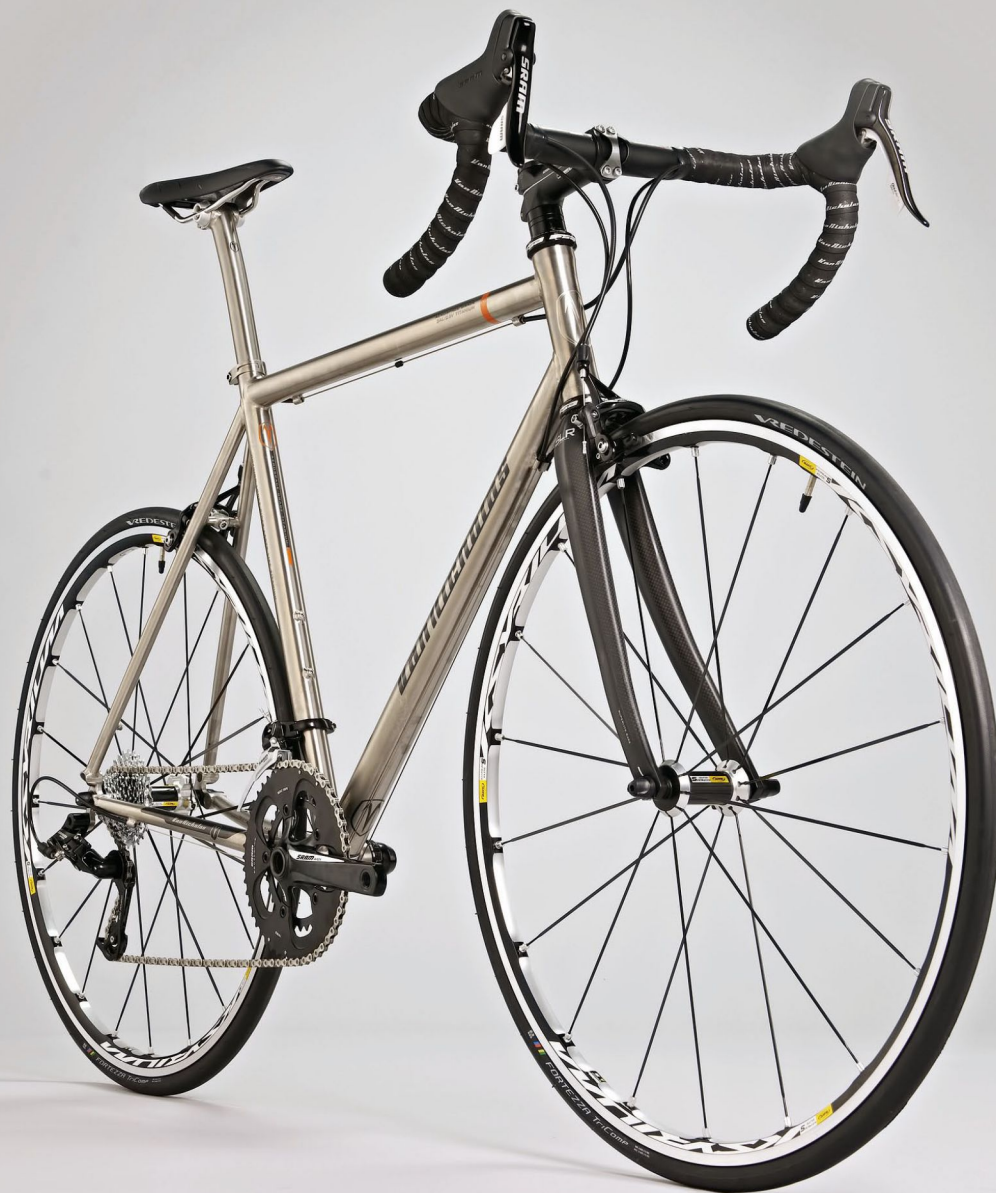
The shortest head-tube here creates a more aggressive riding position
