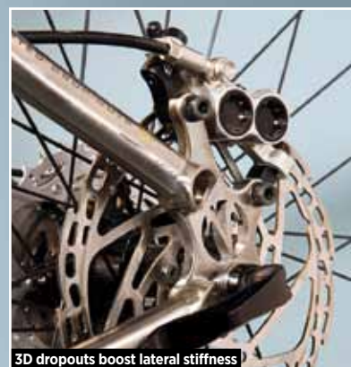
3D dropouts boost lateral stiffness
