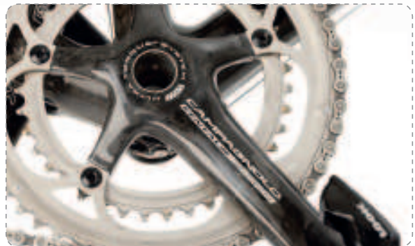
Our Dolan test bike was equipped with a Campag Centaur carbon chainset
