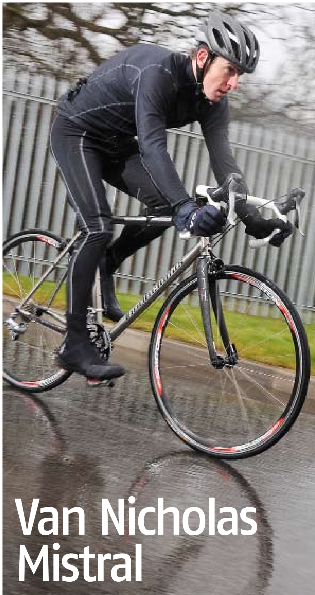
Carbon forks coupled with the titanium frame provide all-day comfort in the saddle.
